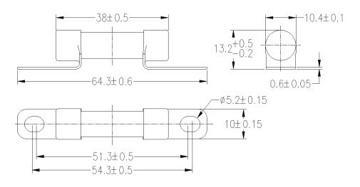
Note: recommend tightening torque is 3.5-4.0Nm.
